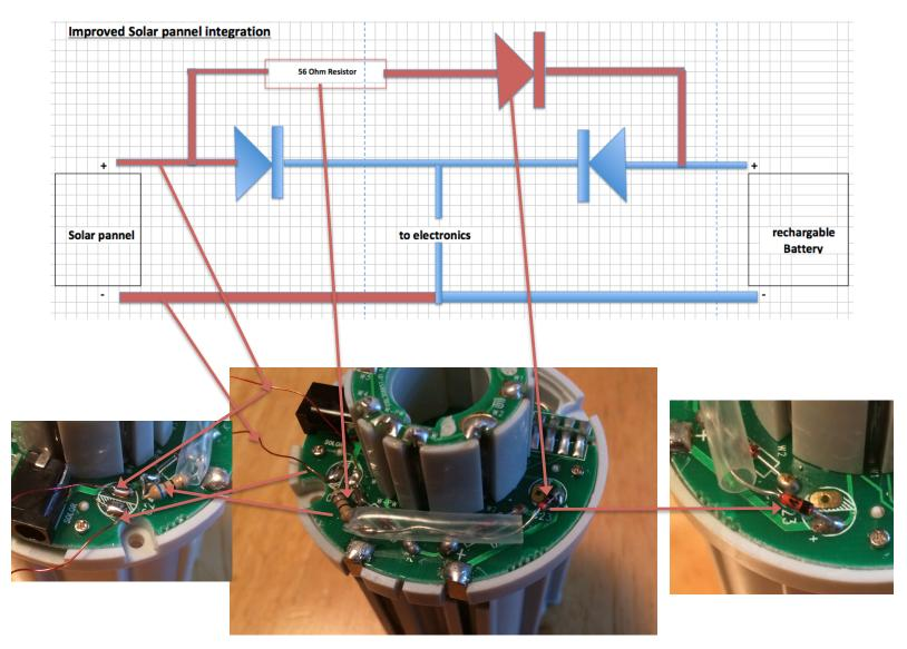
Also: put the diode/resistor into a small heat shrink tube to insulate the blank wires.
