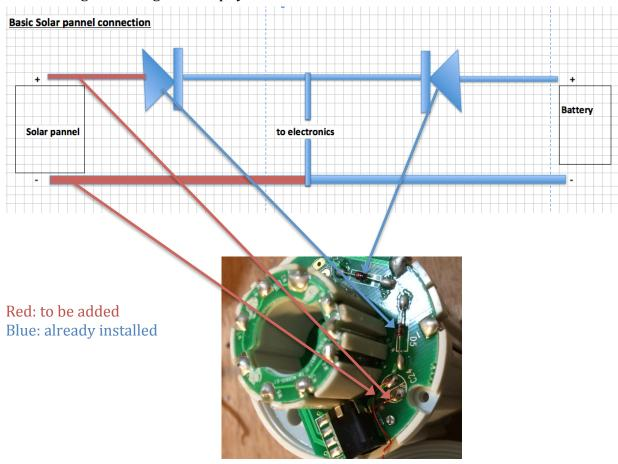
The 2 small wires can be feed through the build in solar panel connector hole:
