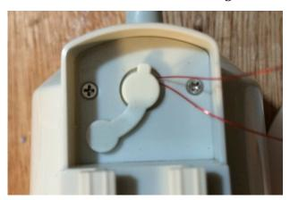
Then solder the wires directly onto the solar panel- remove the old wires that come with the solar panel. You have to connect the wires to the right polarity. If connected with the wrong polarity nothing will happen due to the diode on the board.
