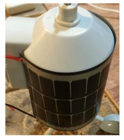
Glue it with superglue around the sensor. It is pretty simple. It fits exactly – it looks as if it was made for THIS purpose! (Actually do this part at the very end. It is easier to open and close the
